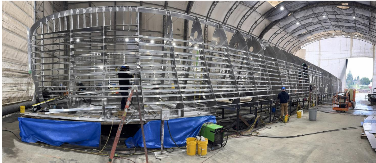
WETA 400 passenger electric ferry fabrication WETA Photo
