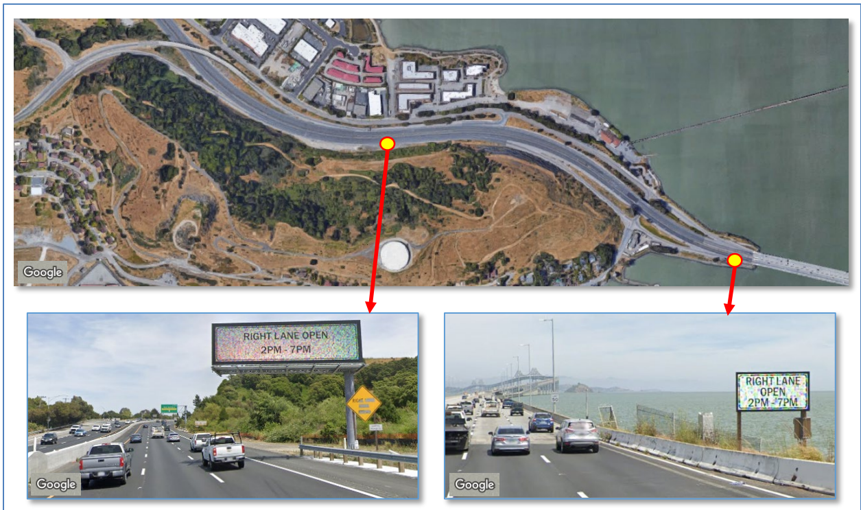
Figure 2-17: Dynamic Sign Indicating Shoulder Open Status
