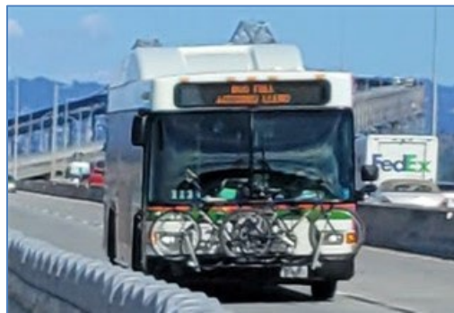
Figure 2-9: Golden Gate Bus Carrying Bikes on Front Rack
