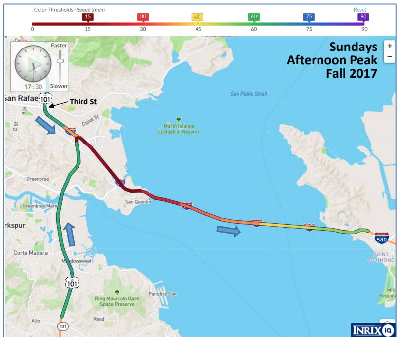
Figure 8-15: Extent of Congestion on I-580 East in Marin County before Bridge Modifications
