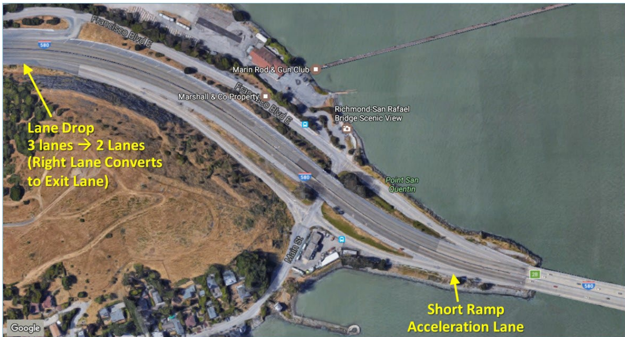
Figure 2-6: Initial Conditions – Eastbound Bridge Approach in Marin County
