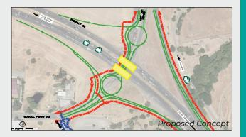
underneath SR 29 to allow for continuous north-south movement of vehicles. The two roundabouts are located on SR 221 north of SR 29 and on Soscol Ferry Road south of SR 29. The roundabouts will accommodate turning movements on and off the highways.
