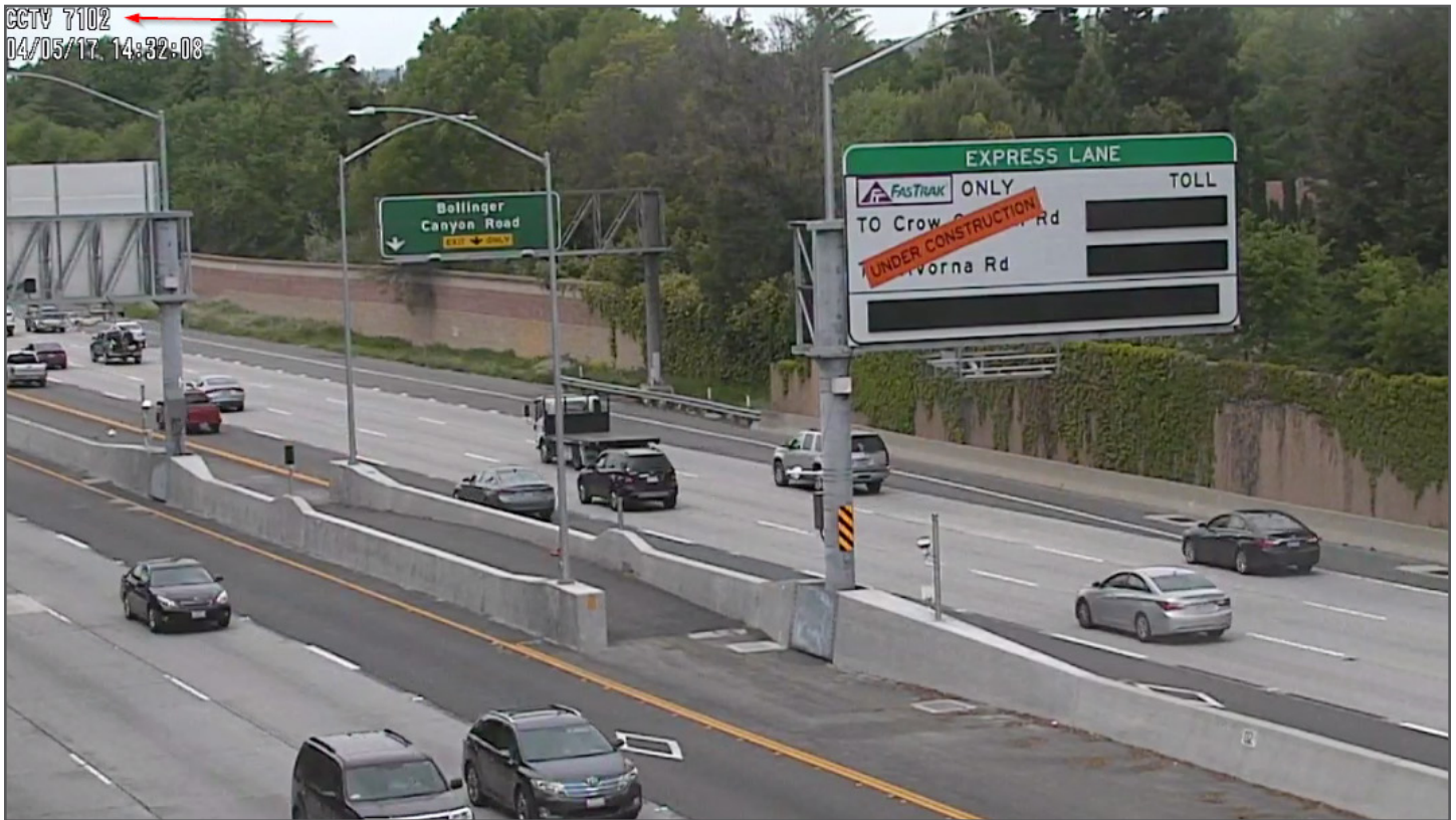
Variable toll message sign at a CHP Enforcement Area on I-680. This screenshot is from a CCTV. The text in the upper left corner indicates the location of the CCTV.
