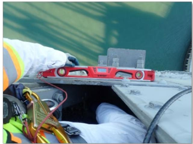
*Figure 1-D: Physically measuring flatness*
