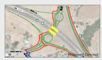
underneath SR 29 to allow for continuous north-south movement of vehicles. The two roundabouts are located on SR 221 north of SR 29 and on Soscol Ferry Road south of SR 29. The roundabouts will accommodate turning movements on and off the highways.
