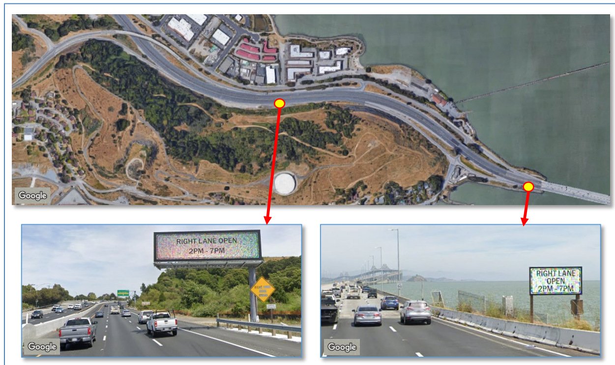
Figure 2-15: Dynamic Sign Indicating Shoulder Lane Open Status
