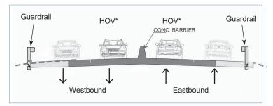
Note: Typical cross section of a four-lane facility is shown. Other project alternatives include part time shoulder running lane, and three-lane contra flow.
